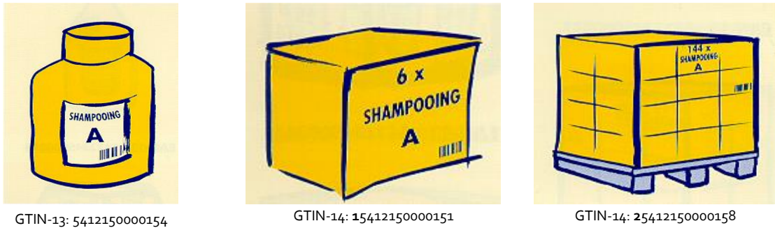
Figure 7-2 Trade item groupings identified with GTIN-14 based on GTIN of consumer unit
